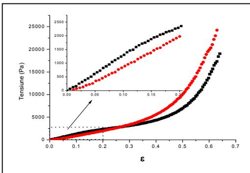
Figure 4. Compression curves for the 50% potatoes paste supplemented bread (■ sample 1; ● – sample 2)
