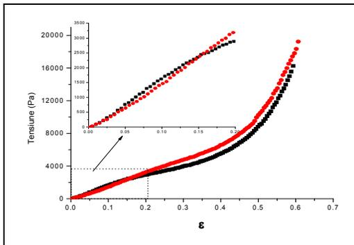
Figure 3. Compression curves for the 30% potatoes paste supplemented bread (■ sample 1; ● – sample 2)
