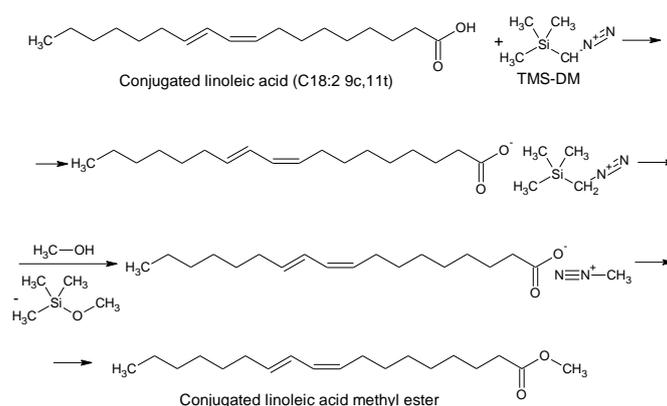
**Figure 6.** Derivatization reaction of the conjugated linoleic acid (C18:2 9c,11t) to the corresponding methyl ester using trimethylsilyl-diazomethane (TMS-DM)
