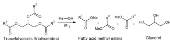
**Figure 4.** Transesterification reaction by boron-trifluoride - methanol of triglycerides to the corresponding fatty acid methyl esters
