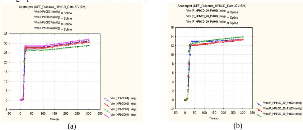
Figure 6. KF water titration curves ( $V/m$  vs.  $Time$ ) for commercial 2-hydroxypropyl- $\beta$ -cyclodextrin (a) and P/2HP- $\beta$ -CD complexes with ethanol 20% (b) – kneading method
