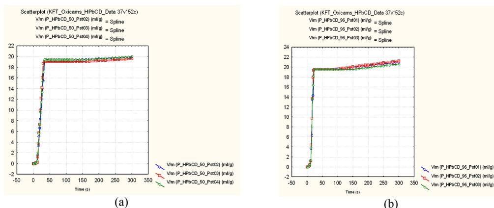
Figure 7. KF water titration curves ( $V/m$  vs.  $Time$ ) for P/2HP- $\beta$ -CD complexes with ethanol 50% (a) and for P/2HP- $\beta$ -CD with ethanol 96% (b) complexes – kneading method
