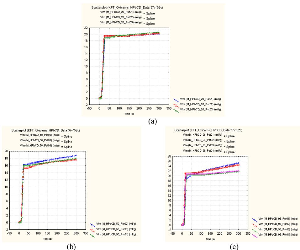
Figure 8. KF water titration curves ( $V/m$  vs.  $Time$ ) for M/2HP- $\beta$ -CD complexes with ethanol 20% (a), for M/2HP- $\beta$ -CD with ethanol 50% (b) complexes and for M/2HP- $\beta$ -CD with ethanol 96% (c) complexes – kneading method
