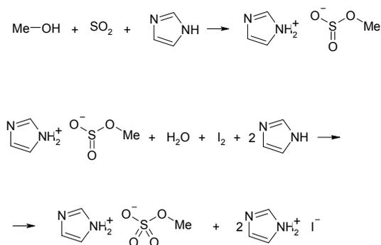
**Figure 2.** Karl Fischer reaction for two-component titration technique
