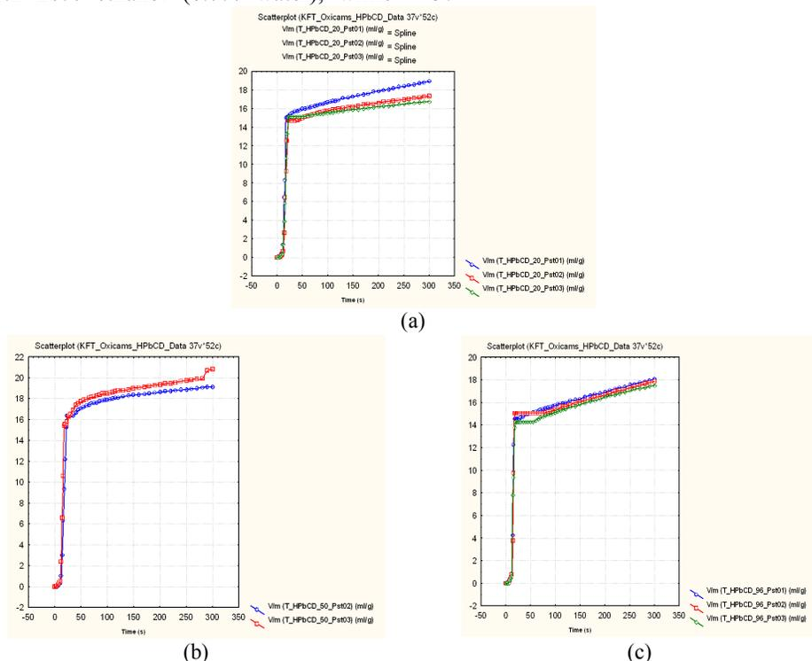
**Figure 9.** KF water titration curves ( $V/m$  vs.  $Time$ ) for T/2HP- $\beta$ -CD complexes with ethanol 20% (a), for T/2HP- $\beta$ -CD with ethanol 50% (b) complexes, and for T/2HP- $\beta$ -CD with ethanol 96% (c) complexes
