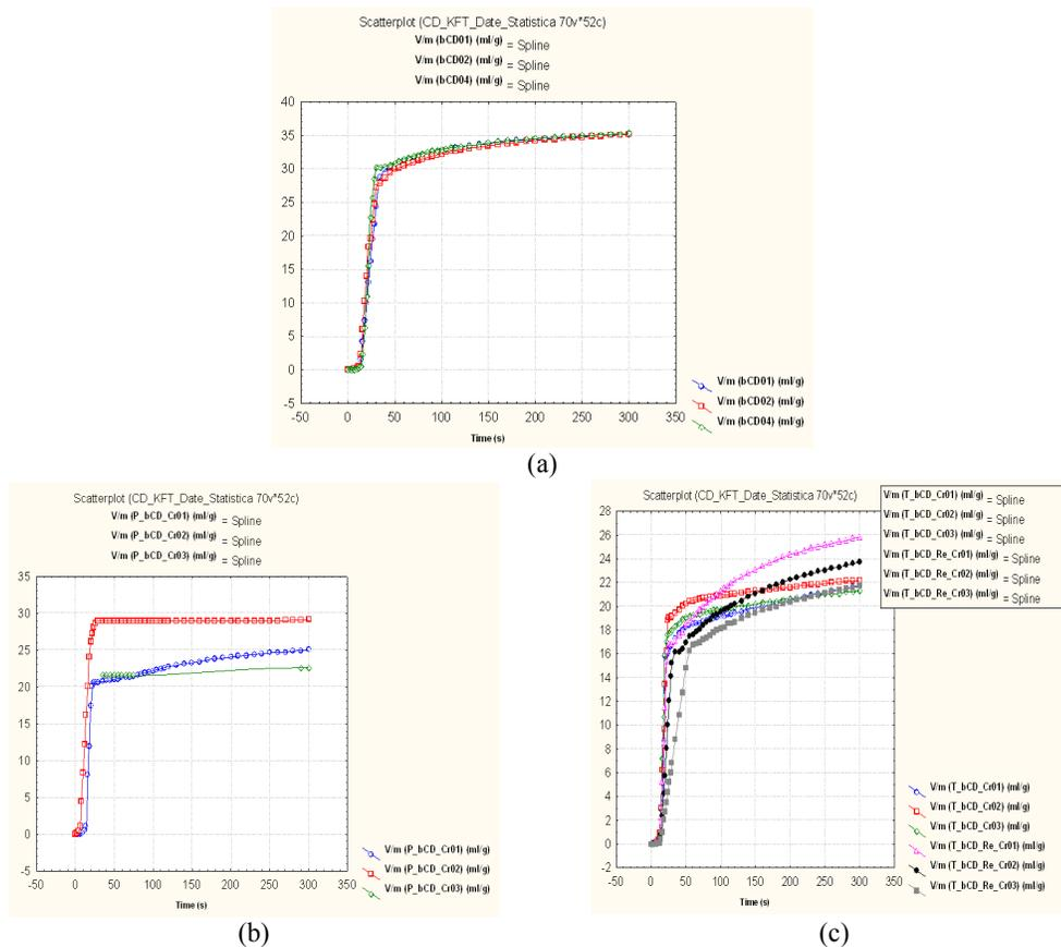
Figure 5. KF water titration curves ( $V/m$  vs.  $Time$ ) for commercial  $\beta$ -cyclodextrin (a), P/ $\beta$ -CD (b), and T/ $\beta$ -CD (c) complexes – crystallization from solution method
