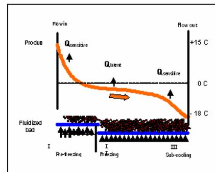
Figure 1. The thermo-dynamic events occurring during the freezing process in fluidized (sursa: IQF Frost)
