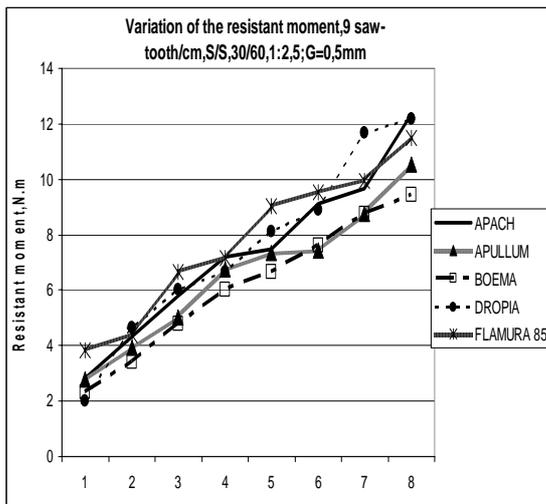
**Figure 2.** The variation of the resistant moment for 9saw- tooth/cm, S/S, 30/60, G=0,5mm roll characteristics.
