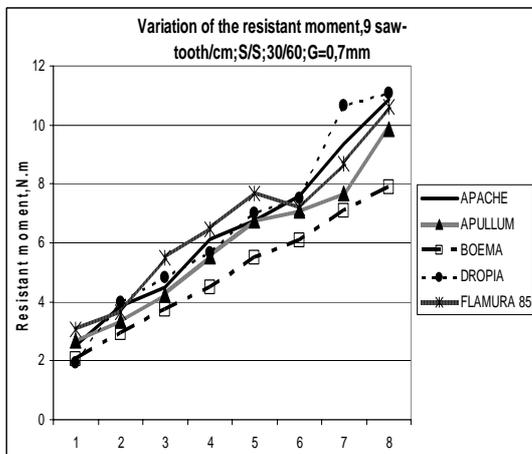
**Figure 1.** The variation of the resistant moment for 9saw-tooth/cm, S/S, 30/60, G=0,7mm roll characteristics
