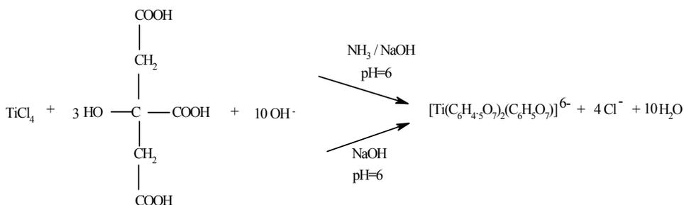
**Fig. 1.** Reactions for the syntheses of  $[\text{Ti}(\text{C}_6\text{H}_4.5\text{O}_7)_2(\text{C}_6\text{H}_5\text{O}_7)]^{6-}$  complex
