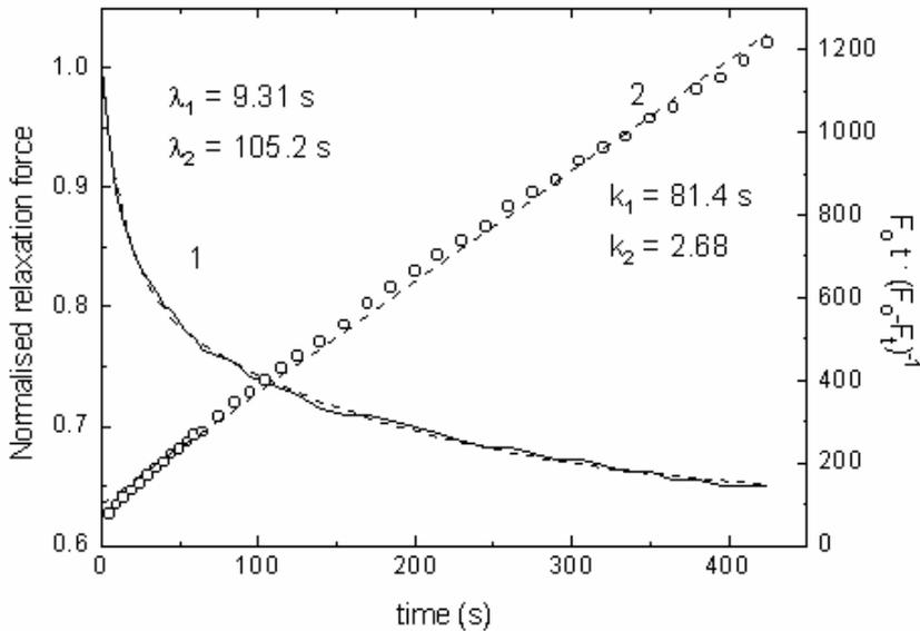
**Fig. 2.** Stress relaxation curves (1) and normalized stress relaxation curve (2) for bread crumb with 0.20% hemicellulose (dot line – calculated curve)
