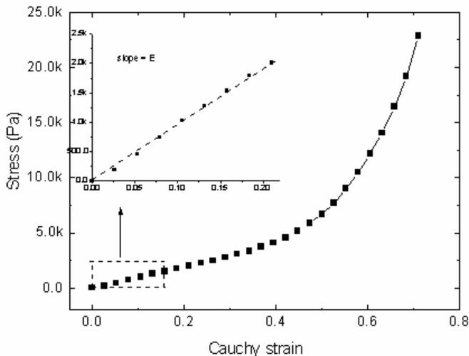
**Fig. 1.** Compression curve for bread crumb with 0.20% hemicellulose
