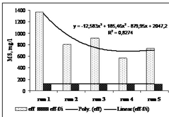
Figure 4. Values of materials in suspension for treated wastewaters into anaerobic stage
