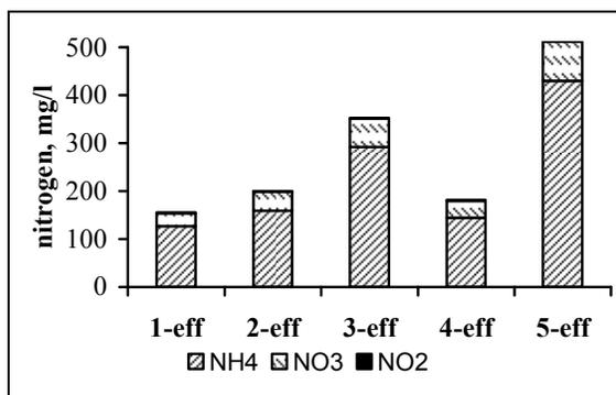
Figure 3. Nitrogen values for treated wastewaters into anaerobic stage
