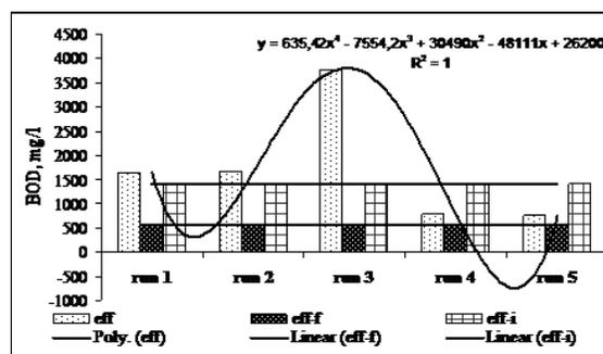
Figure 2. Biological oxygen demand values for treated wastewaters into anaerobic stage
