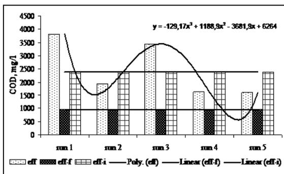
Figure 1. Chemical oxygen demand values for treated wastewaters into anaerobic stage
