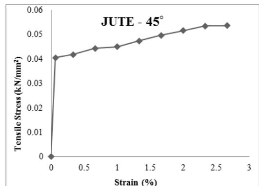
Figura 2. Tensile stress – Strain Curves of the composites reinforced with Jute fabric when tested at (a) $0^\circ$  (b) $15^\circ$  (c) $30^\circ$  (d) $45^\circ$
