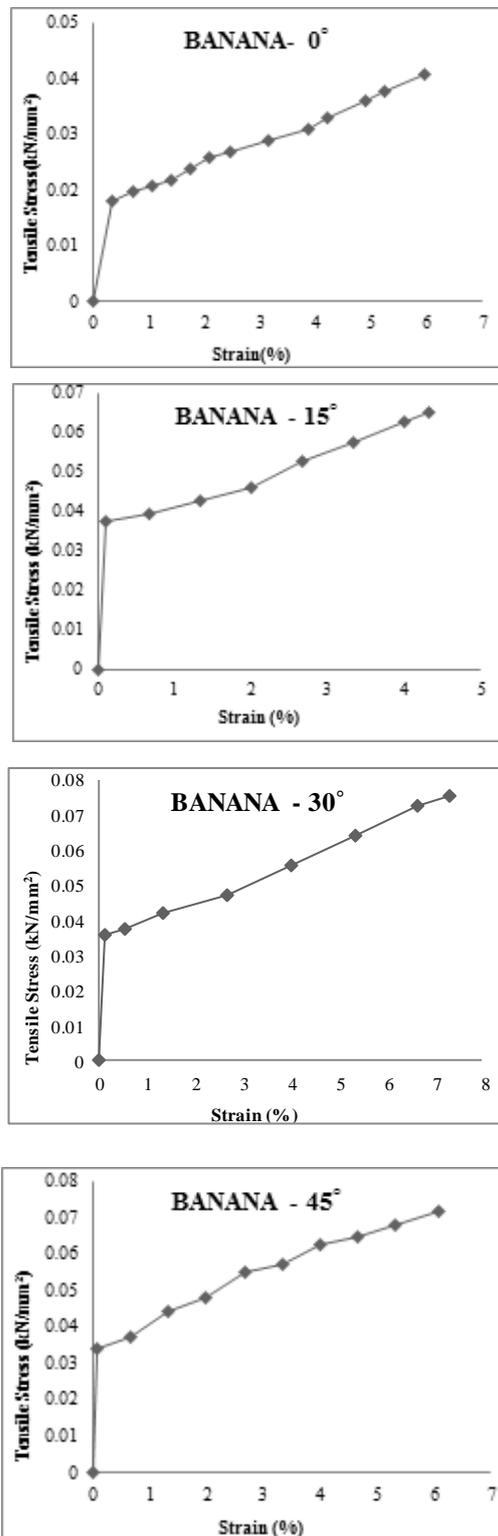
Figure 3. Tensile stress – Strain Curves of the composites reinforced with Banana fabric when tested at (a) 0° (b) 15° (c) 30° (d) 45°
