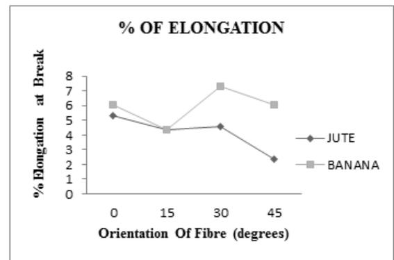
Figure 5. Effect of Test angle on % Elongation of Jute and Banana composite
