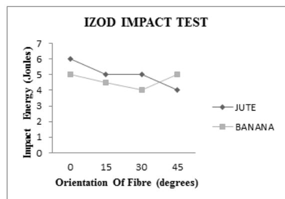
Figure 6. Effect of Test angle on Impact strength of Jute and Banana fiber composite
