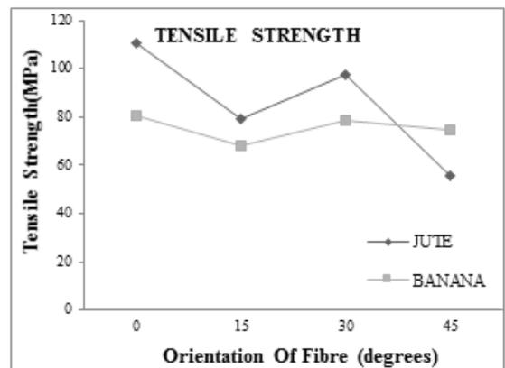
Figure 4. Effect of Test angle on Tensile strength of Jute and Banana composite
