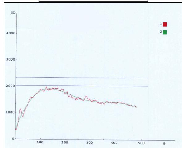
Figure 1. Consistogram for Sample 0 - no added enzyme preparation
