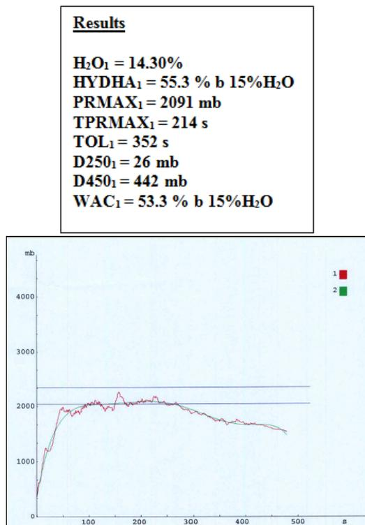
**Figure 2.** Consistogram for Sample 1 – with addition of enzyme preparation based on glucoamylase
