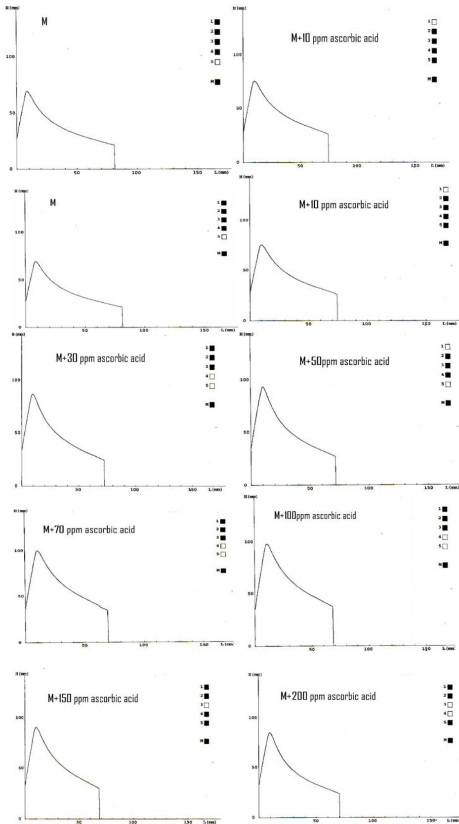
Figure 1. The alveograms for average quality flours (supplemented with different doses of ascorbic acid)
