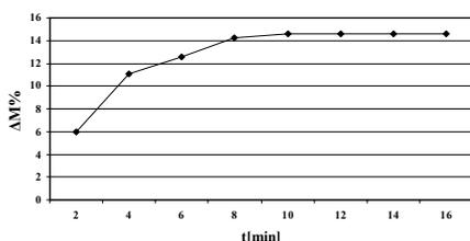
**Figure 2.** The influence of maintaining time under vacuum upon the impregnation of apple
