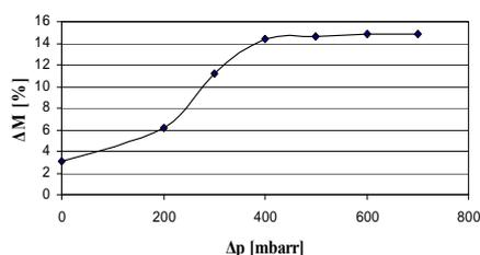
**Figure 1.** The influence of the vacuum's level upon the impregnation of apples
