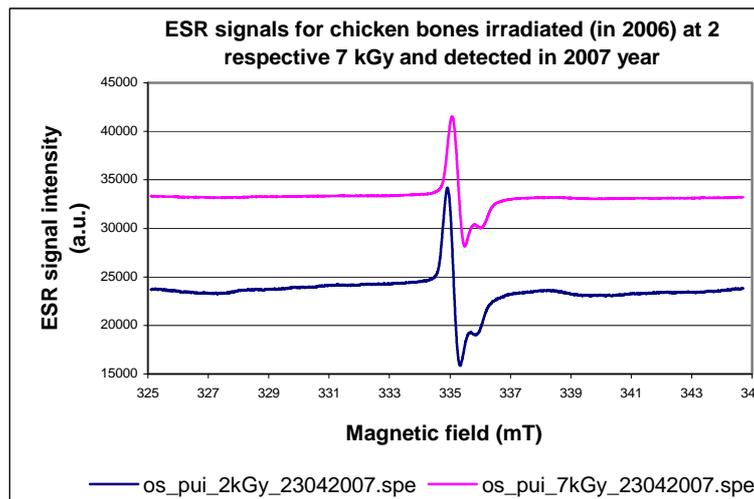
Figure 15 - ESR signal for irradiated chicken bones from 2006 year and detected in 2007 year.
