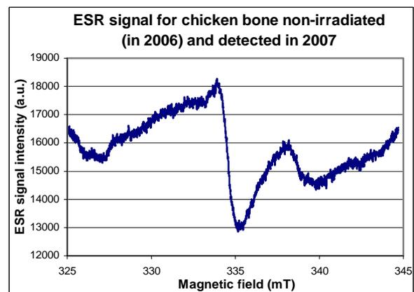
Figure 13 - ESR signal for non-irradiated chicken bones from 2006 year detected in 2007 year.
