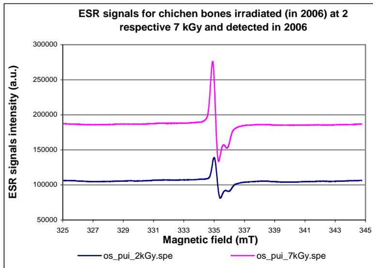
Figure 14 - ESR signal for irradiated chicken bones from 2006 year and detected in 2006 year.
