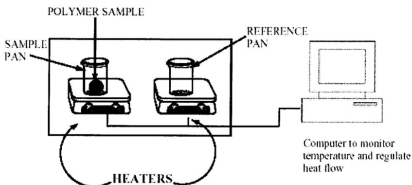
**Fig. 3.** Differential scanning calorimeter ([www.missouri.edu/~crrwww/katti/](http://www.missouri.edu/~crrwww/katti/))
