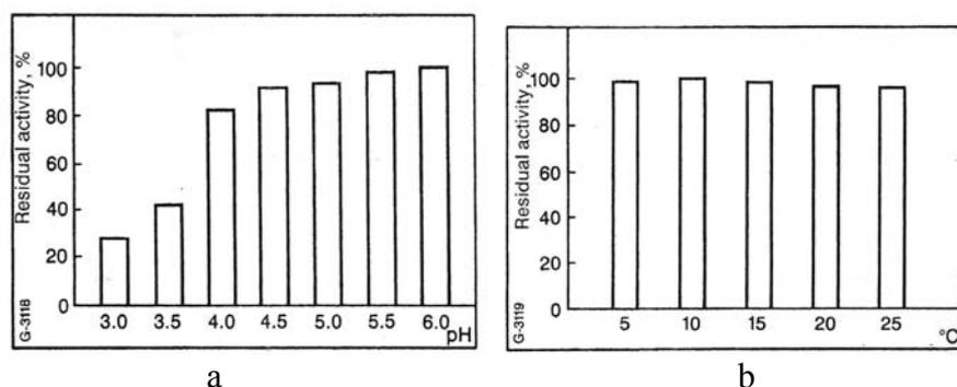
**Figure 3.** The influence of pH (a) and of temperature (b) on the stability of Maturex
