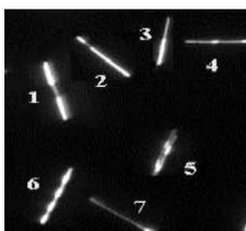
**Fig. 5.** Optical micrograph of a mixture of 7 flavors of Nanobarcodes (<http://www.nanoplextech.com/technology/nanobarcodes.htm>)
