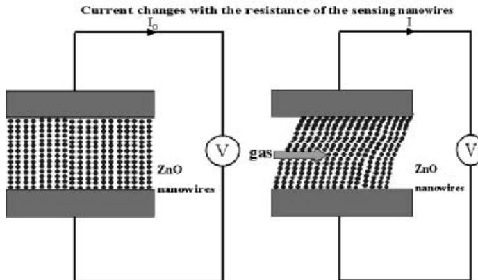
**Fig. 7.** Functional diagram of gas sensors whose current is a measure of change in resistivity of ZnO nanowires on gas adsorption (Chaniotakis, 2004)
