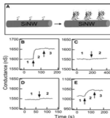
**Fig. 3.** Real-time detection of protein binding (Cui, 2001c)
