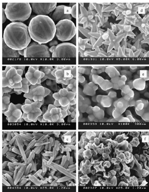
**Fig. 4.** SEM images of calcined ZnO powders (Li, 2003)
