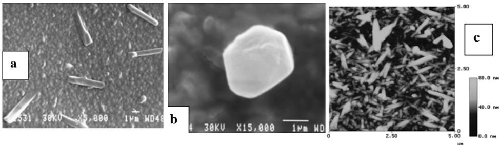
**Fig. 8.** Images of ZnO thin film surface growth from ceramic target by PLD technique: a), b) SEM, c) AFM. (Suchea, 2005)
