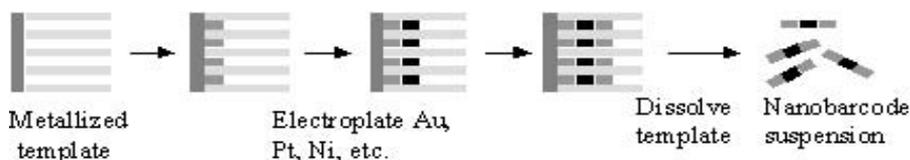
**Fig. 6.** Template-directed synthesis of Nanobarcodes particles (<http://www.nanoplextech.com/technology/nanobarcodes.htm>)
